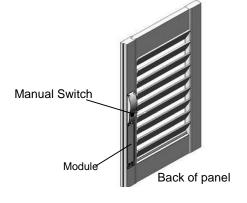
TOOLS needed: Pliers, Phillips head screwdriver and a small coin
