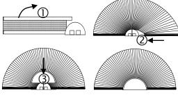
For Quarter Round, Arch on Top, Angle Top, and Half Eyebrow (take Quarter Round as example): Open the shade and place the rail into the bottom of 90° center support tightly, and then install the front and
