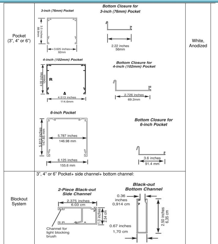
Important Note: The size of Fascia and Cassette is determined by the manufacturer based on the tube and clutch size. 5" Square Fascia is for dual shades only. If Galaxy clutch is specified, Cassette, Cassette with fabric insert and Rounded Fascia are not available.
